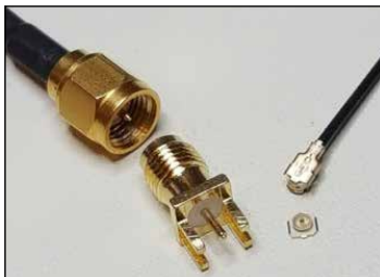
▲ Fig. 4 The UFL micro-cox connectors and lead wires require much less circuit board space than the more common SMA connectors. The micro-coax is a good solution for compact spaces.
