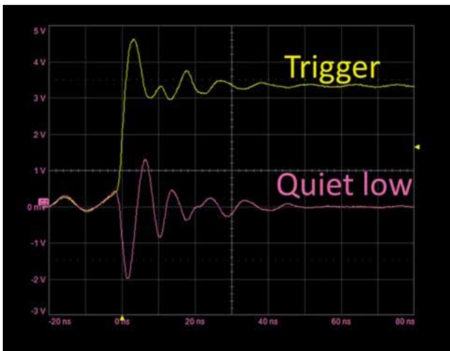
▲ Fig. 3 Signals from the student board measured with a Teledyne LeCroy HDO8108 scope showing a peak-to-peak ground bounce of more than 3 V.
