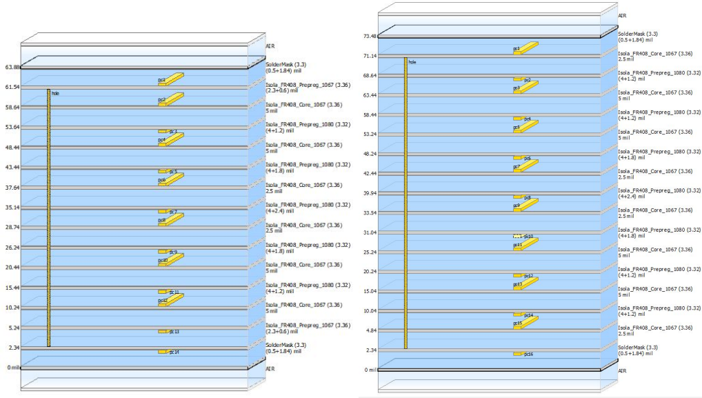
Figure A.9 - Definition of 14L PCB Stack-up (left) and 16L PCB Stack-up (right)
