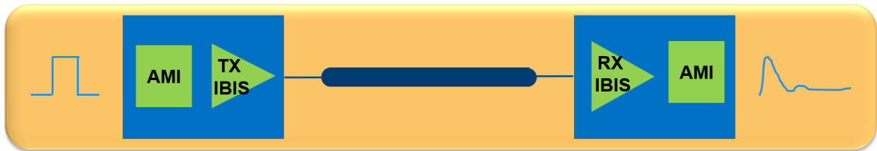
Figure 13: IBIS-AMI GetWave simulation flow.
