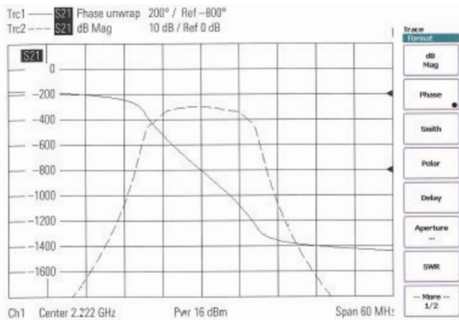
Fig. 4.5.3 Phase and magnitude curve for a bandpass filter.
