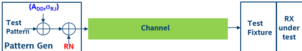
Fig.1-b Interference tolerance Test Setup for 100GBASE-CR1, etc.
