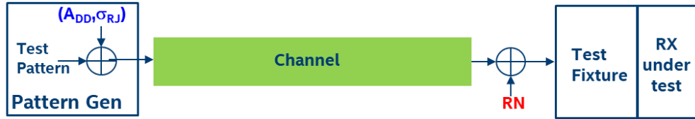
Fig.1-a Interference tolerance Test Setup for 100GBASE-KR1, etc.
